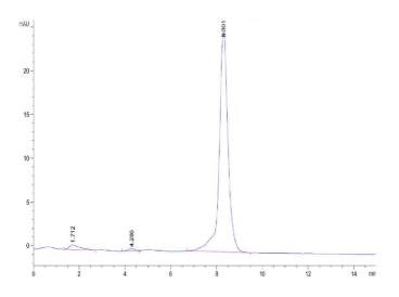
The purity of Human FSH alpha&beta is greater than 95% as determined by SEC-HPLC.
