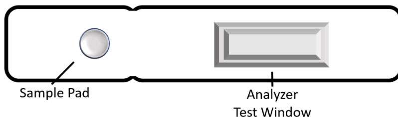
Figure 1: Schematic of the Cassette with labeled Sample pad and Analyzer Test Window Sections
