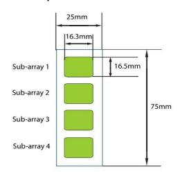
4 printed sub-arrays per glass chip
