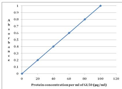
Legend: The standard curve shown in Fig. 1 represents the average absorbance reading of several common proteins (e.g., actin, BSA, casein) measured in a 1 ml cuvette format using 1 ml of GL50 reagent. The protein reading pathlength for a cuvette is 1 cm. Linear range of this assay is 0.05 - 0.6.
