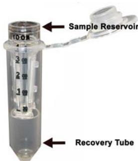
2. Apply 0.5 mL of the recovered AAV fraction (step 18 above) to the sample reservoir of the Centrifugal Concentrator. Cap the concentrator and place into a tabletop microcentrifuge. Centrifuge for 5 minutes at 2,000 x g. Flow through can be discarded.
