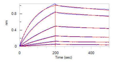
Loaded SARS-CoV-2 S protein RBD, Fc Tag (Cat. No. SPD-C5255) on Protein A Biosensor, can bind Cynomolgus ACE2, His Tag (Cat. No. AC2-C52H7) with an affinity constant of 4.48 nM as determined in BLI assay (ForteBio Octet Red96e) (Routinely tested).
